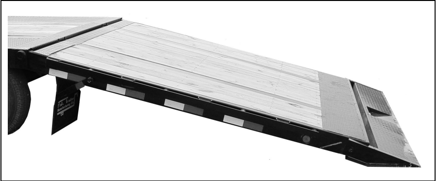
Dovetail Lowered – Figure 6-5
